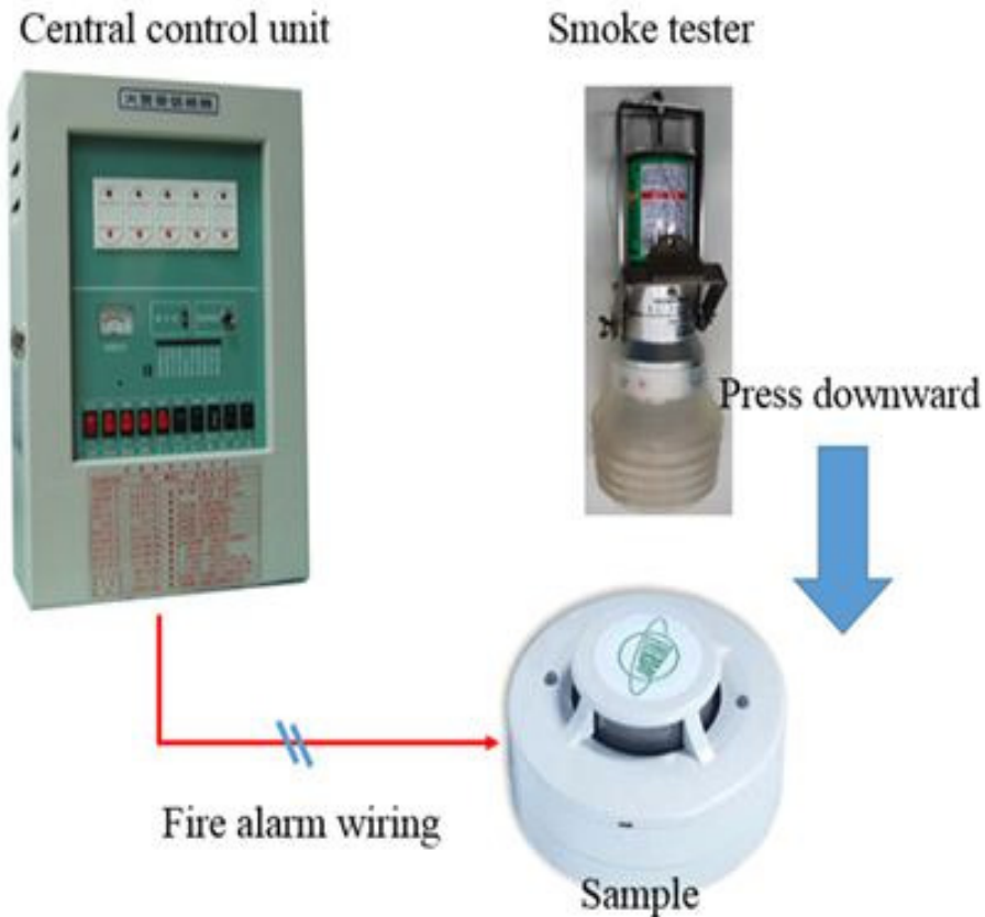
Figure.3 Method used to test sample via smoke tester
