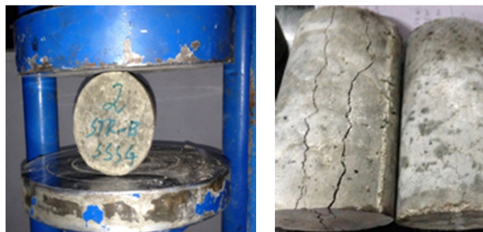
Figure 5. Split tensile strength of cylinder
