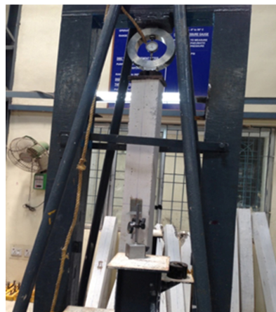
Figure 6. Loading frame for testing the column
