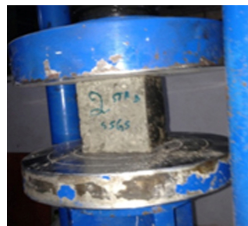
Figure 4. Compression testing on cube
