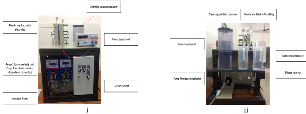
Figure 1 The front (i) and the rear view (ii) of the electrodiagnosis unit
