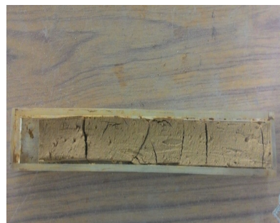
Fig. 1b. Linear shrinkage (14 days)
