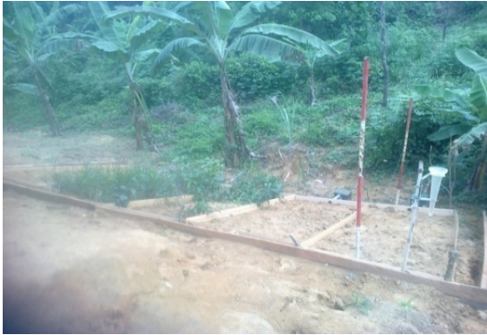
Plate 1: Researchers' Experimental Plot with Ranging Poles and Rainguage
