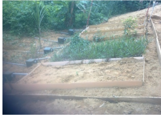
Plate 2: Researchers' Experimental Plot with Sedimentation Boxes
