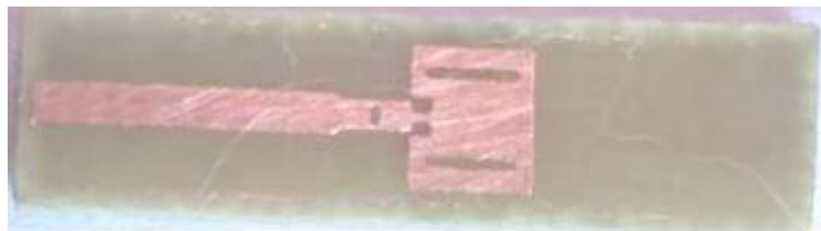
Figure 5: A fabricated prototype of the proposed antenna
