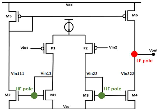
Fig. 4. Operational Amplifier of the bandgap voltage reference
