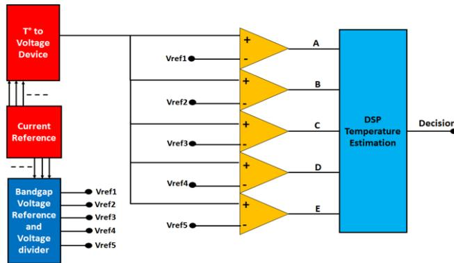
Fig. 2. Architecture of the stand-alone temperature monitor
