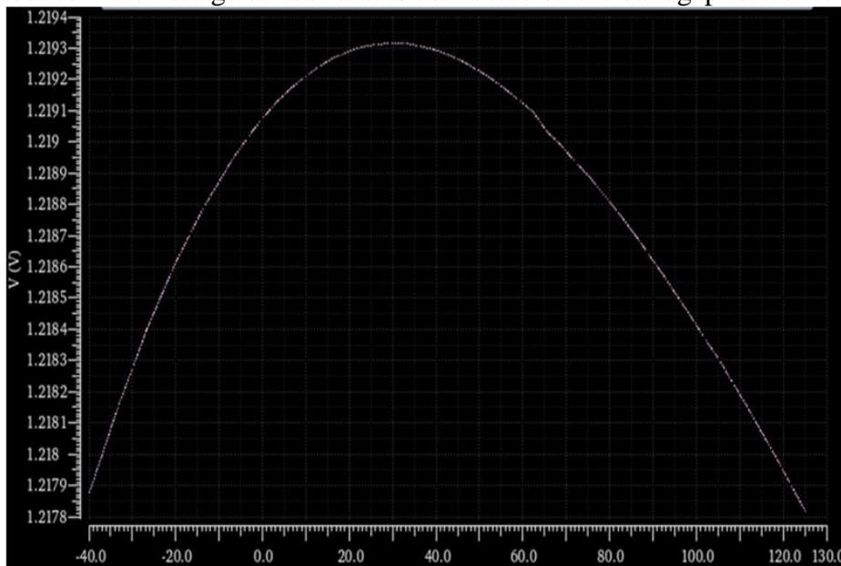
Fig. 9. Bandgap voltage reference output variation with the temperature
