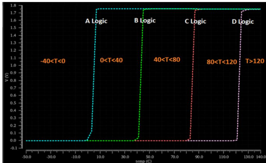
Fig. 10. Comparators outputs depending in terms of the chip temperature
