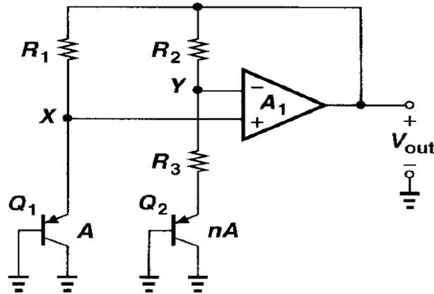
Fig. 3. Bandgap Voltage Reference [1]
