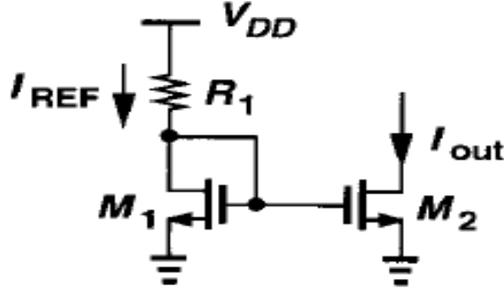
Fig. 5. Current reference using simple resistor [1]
