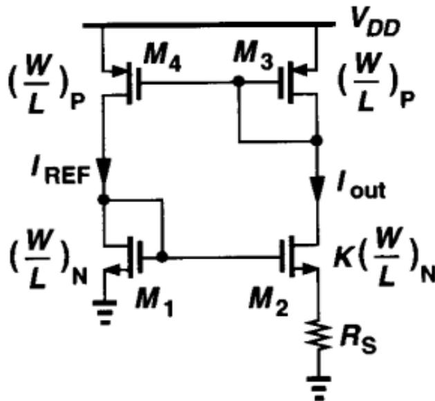
Fig. 6. Supply Independent Current Reference [1]
