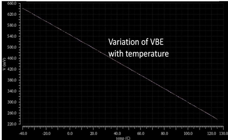
Fig. 8. Variation of the sensing device output with the temperature
