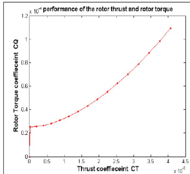
The curve gives an indication that the relation between the thrust and the torque coefficient is almost linear.
