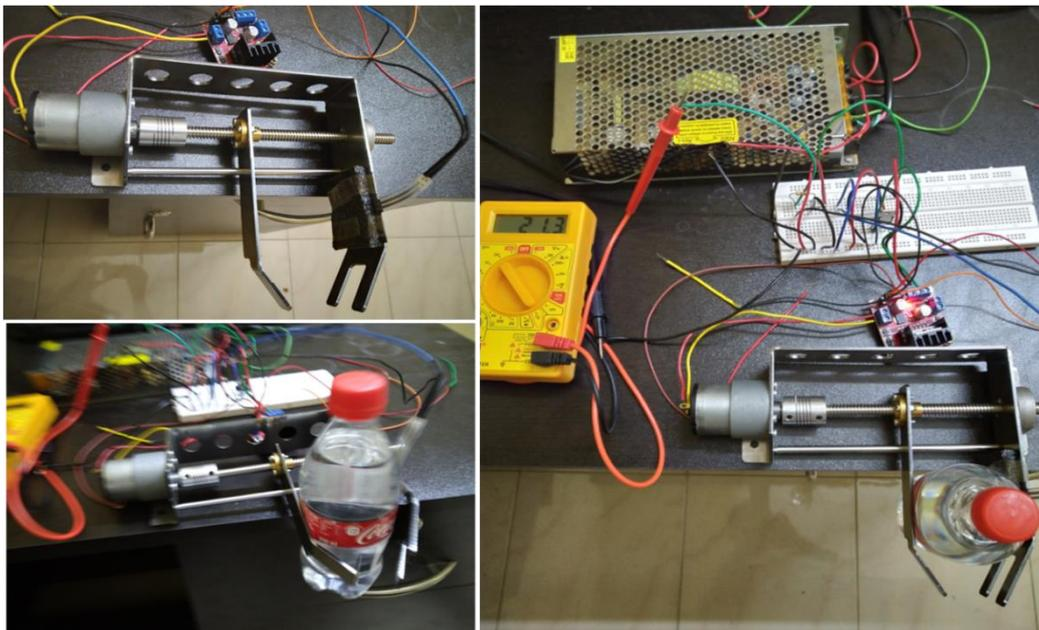
Figure 10. L.S.Gripper assembly operation
