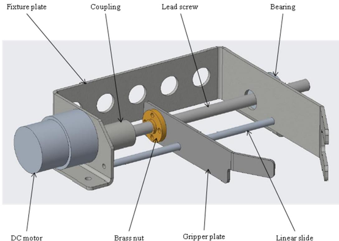
Figure 1. CAD assembly model of l.s.gripper
