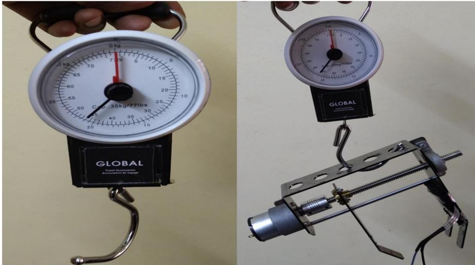
Figure 11. Analog weighing scale & gripper weight measurement
