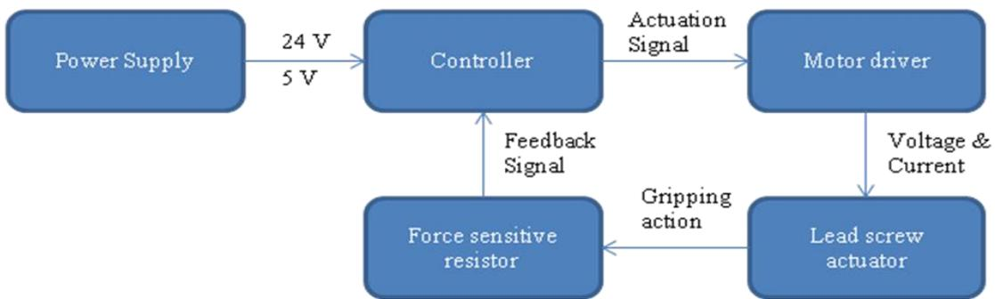
Figure 4. Mechatronic system concept for the l.s.gripper
