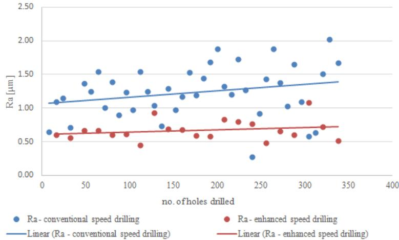
Figure 7 Surface roughness (Ra) after drilling 338 holes
