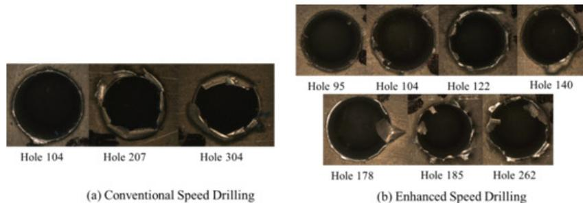
Figure 8 Exit burr formation on both work piece
