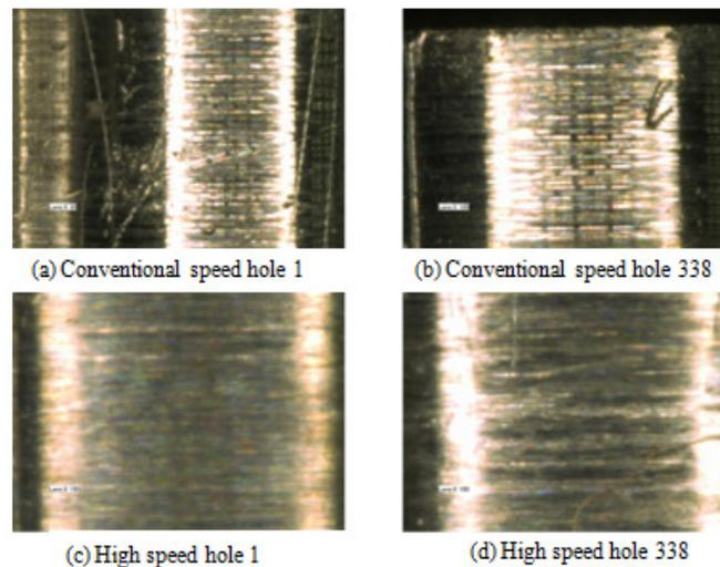
Figure 6 Cutaway view magnification drilling holes
