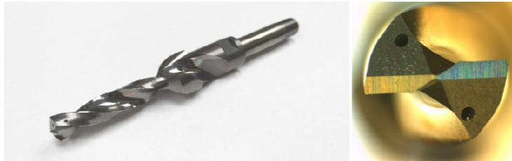
Figure 1 (a) Twist carbide drill tool utilised in this experiment (b) top view
