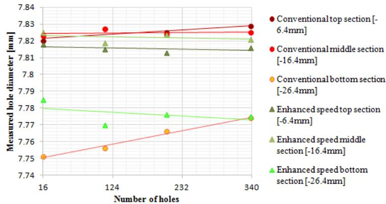
Figure 5 Measured diameter of the holes on different depths from both cutting speeds at different life stages (hole 16, 112, 208, and 338)
