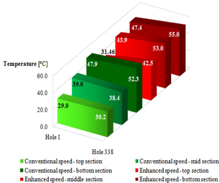
Figure 4 New tool and worn tool drilling temperature measured at both cutting speeds
